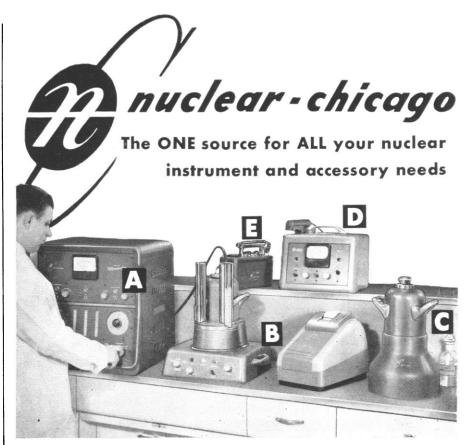
This radiation counting laboratory includes: A—Scaler, B—Automatic Sample Changer, C—Scintillation Well Counter, D—Count Rate Meter, E—Portable Survey Meter, all made by Nuclear-Chicago.
