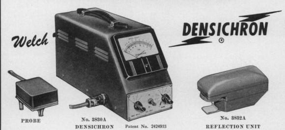
The Welch Densichron is an electronic densitometer of good sensitivity and unusually high stability. It can be employed either for quantitative measurement of optical density, or as a sensing device for automatic control of various industrial processes in which constancy of transmitted or reflected light is a criterion of the quality or uniformity of the product.
