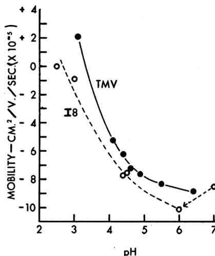
Fig. 3. Electrophoretic mobility of concurrently isolated preparations of I8 and TMV at various  $\text{pH}$ 's. All samples were dissolved in buffers of ionic strength 0.1, which contained NaCl to provide common ions (4).
