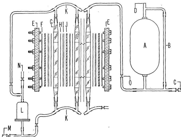
Fig. 1. Schematic diagram of assembled ultrafiltration apparatus. Filter unit is shown in exploded view: *A*, reservoir (3); *B*, level gauge; *C*, reservoir inlet; *D*, compressed gas inlet; *E*, end plate; *F*, rubber pad; *G*, Cell; *H*, membrane (4); *I*, filter paper (5); *J*, filter plate (6); *K*, manifold; *L*, receiving flask (7); *M*, concentrate tap; *N*, air bleeder; *O*, screw clamp.
