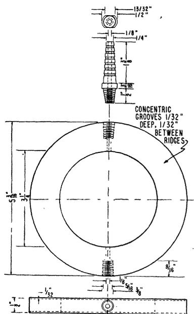
Fig. 2. Details of Plexiglas cell.
