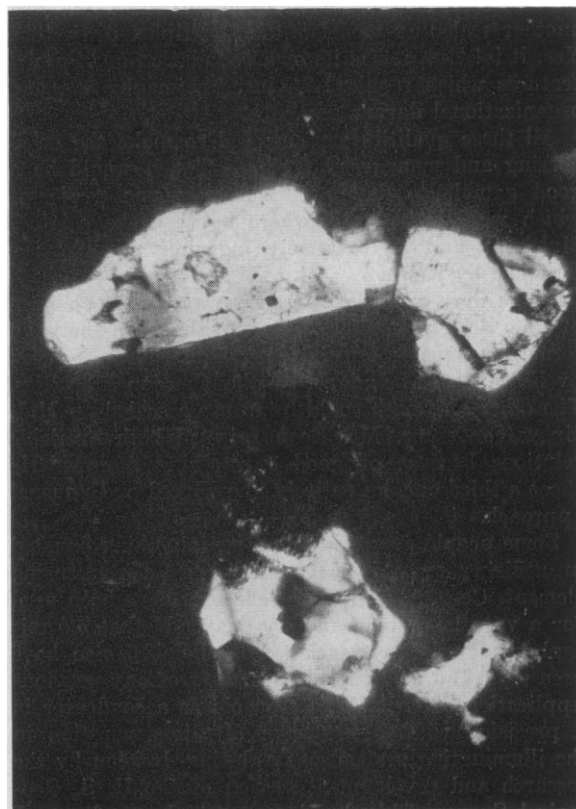
FIG. 2. Dust particles collected on a Millipore filter and sectioned in plastic. Transmitted illumination, crossed nicol prisms. 150 x.
