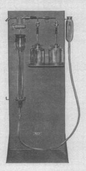
A modified Haldane gas analysis apparatus used to demonstrate the technique of gas analysis in student teach-
