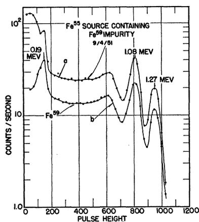
FIG. 1. Pulse height spectrum of  $\text{Fe}^{55}$  and  $\text{Fe}^{59}$   $\gamma$ -rays.
