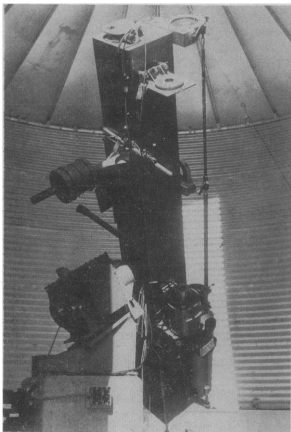
FIG. 6. Sacramento Peak flare recorder mounted on the 10-foot spar.
