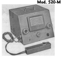
For the exact measurement of extremely low light values down to 1/10,000 microlumen.
