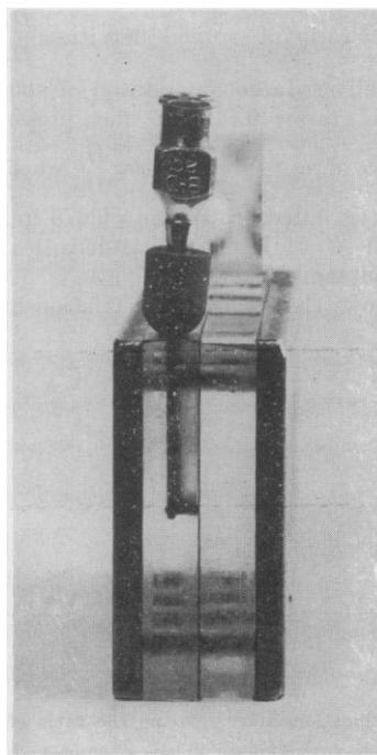
FIG. 2. Side view of cuvette with filling needle in place.
