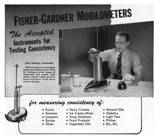
The Improved Fisher-Gardner Mobilometer enables determinations of mobility by observing the time required for a standard disc to descend a fixed distance through a sample.
