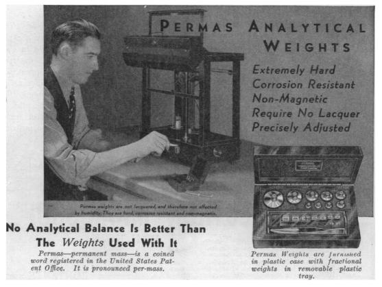
Permas Weights have physical properties which enable them to serve better than gold-plated, platinum-plated, or lacquered brass weights in the analytical lab-oratory. They retain their carefully-adjusted mass much longer than weights made of other metals.
