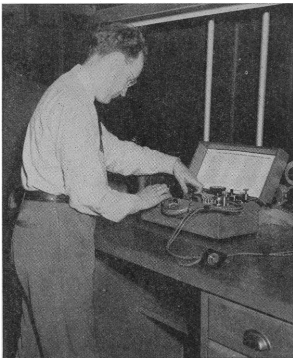
Measuring resistance across the contact in a Spencer Thermostat element, by means of L&N Kelvin Bridge.
