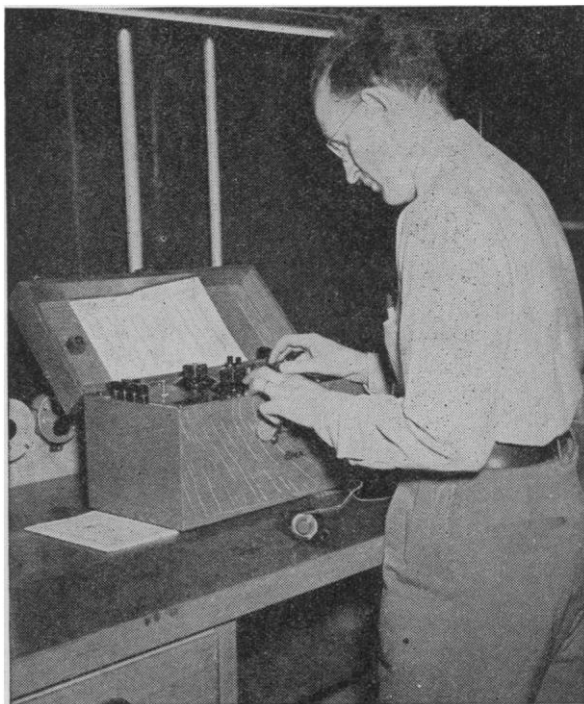
Measuring temperature of thermocouple inserted in Spencer Thermostat by means of an L&N Precision Portable Potentiometer.
