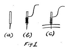
red in a Bunsen flame for a few seconds lose their brittleness. The needle then is wrapped tightly with fine copper or silver wire from the lower part of its thickened shank to within about 5 mm of its top (Fig. 1b). It is well to let one end of the coiled wire extend for several inches from the shank so that clips connected to the recording apparatus can later grip the wire, thus making a flexible, non-rigid connection which will prevent pull on the implanted elec-
