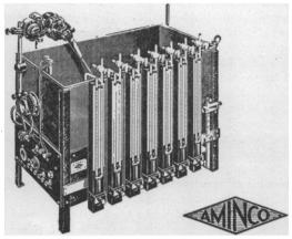
For all temperatures from  $-20^{\circ}$  to  $100^{\circ}$  C., with thermoregulator control to  $\pm\,0.05^{\circ}$  C. (or closer).
