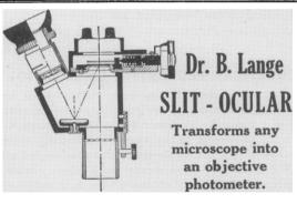
For photometric measurements of spectral and X-ray photos, determination of light-absorption of micro specimens and colorimetric determination of fluids in layer thicknesses from 0.1 mm. Direct reading of absolute density and light permeability values on dual scales of Multiflex Galvanometer.
