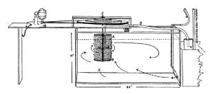
in the accompanying illustration. Strong circular currents are formed in the immediate vicinity of the cylinder, while at the far end the water moves very gently. There is also a noticeable upward motion from the bottom of the tank.
