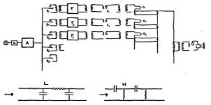
"M'' is condenser microphone with associated small amplifier (a) leading to the larger boosting amplifier (A). "R''s are repeater tubes which avoid throwback on the primary circuit—thus making it possible to use one or all filters ("F''s) separately or simultaneously. "X''s are tubes operating oscillographic units ("O''s). The last part of the circuit is an arrangement for synthesizing the analyzed currents. "L'' and "H'' refer to general type filter circuits (resistance and capacitance).
