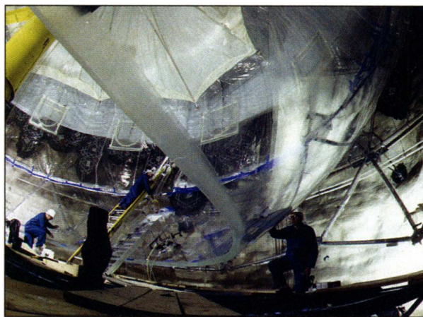
Positive ID. A huge sphere of heavy water caught fugitive neutrinos as they changed from one flavor to another.
