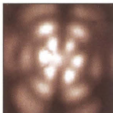
Emission patterns of coupled lasers, at two injection currents and pulse lengths.
