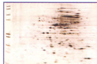
Protein spots from E. coli lysate separated in the first dimension by IEF using ZOOM ® IPGRunner ™ and in the second dimension by SDS PAGE on NuPAGE ® ZOOM ® gel.
