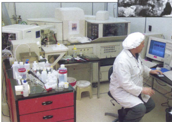
Nuclear sleuthing. Livermore scientists used the IsoProbe, a state-of-the-art mass spectrometer, to precisely measure radioactive isotopes and impurities in a uranium sample seized by Bulgarian border guards. An electron microscope revealed unusually fine grains of uranium oxide, like this sample ( inset ).
