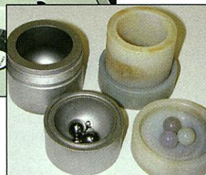
Dry chemistry. Milling machine (above) triggers reactions by shaking organic powders in vials with steel balls.
