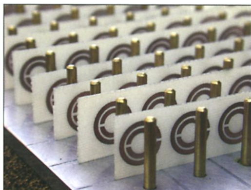
Weird stuff. Researchers say this "metamaterial" can refract microwaves the wrong way.
