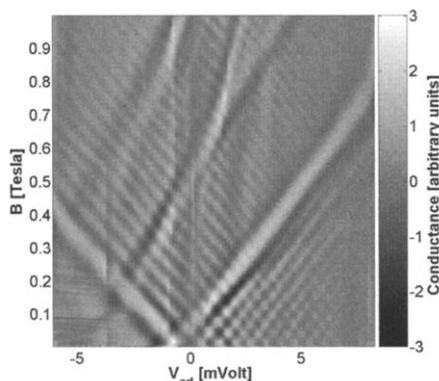
**Fig. 4.**  $G(V_{sd}, B)$  for a 2- $\mu\text{m}$ -long tunnel junction at low  $B$ . A smoothed background has been subtracted to emphasize sharp features, although these are quite clear in the raw data. Oscillations are seen off the dispersion curves, several of which are easy to see.
