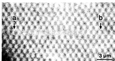
**Fig. 4.** Disappearing images of more vortices in a single chain ( $T = 57$  K,  $B_{\perp} = 0.8$  mT,  $\theta = 80^{\circ}$ ). We attribute the disappearance of the vortex images to the synchronous oscillation of vortices between the node vortices a and b along the chain direction, just like a coupled oscillation.
