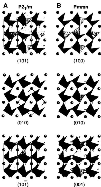
**Fig. 3.** Possible crystal structures of  $\text{MgSiO}_3$  perovskite above 83 GPa. (A)  $P2_1/m$  and (B)  $Pmmn$ . Projections along pseudo-cubic axes are shown for comparison. The crystal structures of  $P2_1/m$  and  $Pmmn$  have same tilting senses as  $Pbnm$  and  $P4_1/nmc$ , respectively. The unit cell is shown by solid lines.
