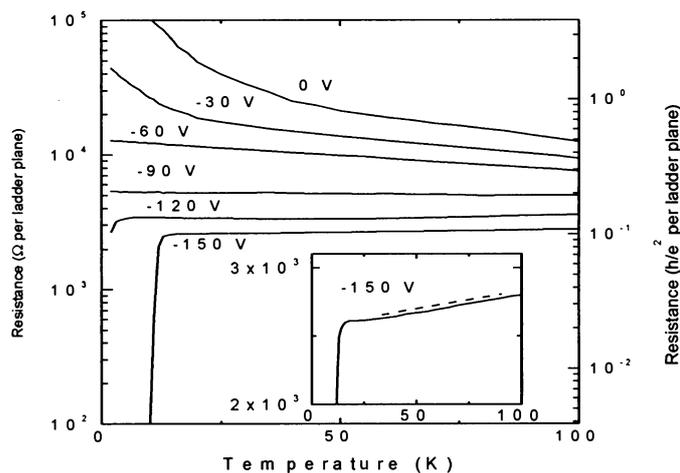
**Fig. 4.** Resistance per ladder plane of a  $[\text{CaCu}_2\text{O}_3]_4$  film as a function of temperature and the applied gate bias. A transition from insulating to metallic and, finally, to superconducting behavior is observed. The inset shows the resistance at  $-150$  V on a linear scale. The dashed line corresponds to a linear dependence.
