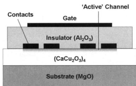
**Fig. 2.** Field-effect device structure. The  $[\text{CaCu}_2\text{O}_3]_4$  film is grown by MBE on a MgO substrate. Electrical contacts are prepared on top of the film by thermal evaporation. An  $\text{Al}_2\text{O}_3$  insulating layer is deposited by sputtering. Finally, a gold layer is evaporated as gate electrode.
