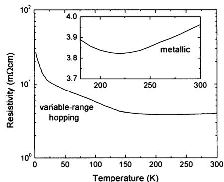
**Fig. 3.** Resistivity per ladder plane of an as-grown  $[\text{CaCu}_2\text{O}_3]_4$  film as a function of temperature. Below 150 K, the transport is governed by variable range hopping. Above  $\sim 220$  K, metallic behavior is observed (see inset).
