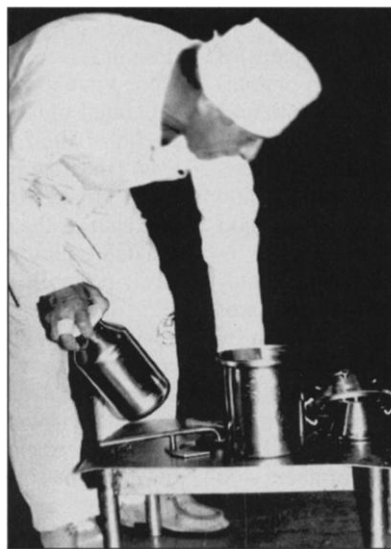
Portability of separated plutonium. The canister held by this worker in Russia's commercial reprocessing complex near Chelyabinsk contains 2.5 kg of plutonium dioxide powder. The material in three of these easily portable containers would suffice to make a nuclear explosive. The complex's warehouses contain over 13,000 such containers.
