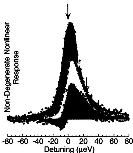
Fig. 4. Nondegenerate ( $\Omega_1 \neq \Omega_2$ ) spectral mapping of a single eigenstate. Each spectrum represents a different spectral position of the pump ( $\Omega_1$ ), which is indicated by the arrow.
