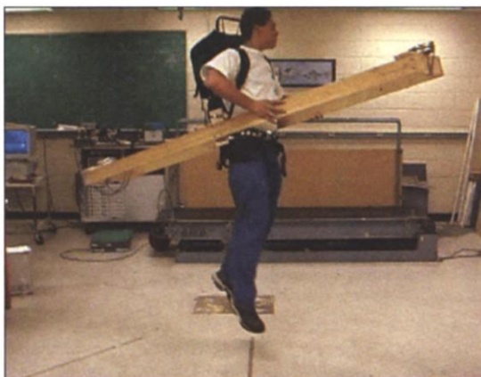
New twist. Experiments with a weighted frame show that some large dinosaurs had trouble turning.
