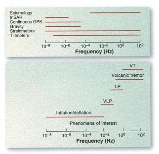
**Toward volcanic prediction.** Various ground-motion measurement techniques and the corresponding phenomena that can be studied with a variety of instrumentation. VT, volcano-tectonic; VLP, very-long-period; and LP, long period events.
