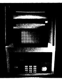
The GeneAmp® PCR System 9700 is available with a gold-plated silver 96-well sample block or with an AutoLid-enabled dual 384-well sample block.
