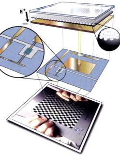
The nuts and bolts of electronic paper. The exploded view shows the elements in a unit cell (not to scale). Arrays of rubber-stamped plastic transistors (inset on the left; blue, organic semiconductor; gold, source/drain electrodes; gray, gate electrode) control the color of a layer of microencapsulated electronic ink (inset on the right).
