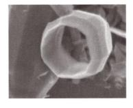
were grown under hydrothermal conditions. Electron microscopy reveals that carbon nanotubes seed the growth of several radially joined, highly ordered graphite crystals. These crystals have diameters up to 1 micrometer, and their faces, which are remarkably equal, range in number from 7 to 14. They also show high conductivity and mechanical strength.
