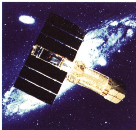
Premature ending. Solar storm increased atmospheric drag on ASCA, sending the spacecraft spinning out of control.
