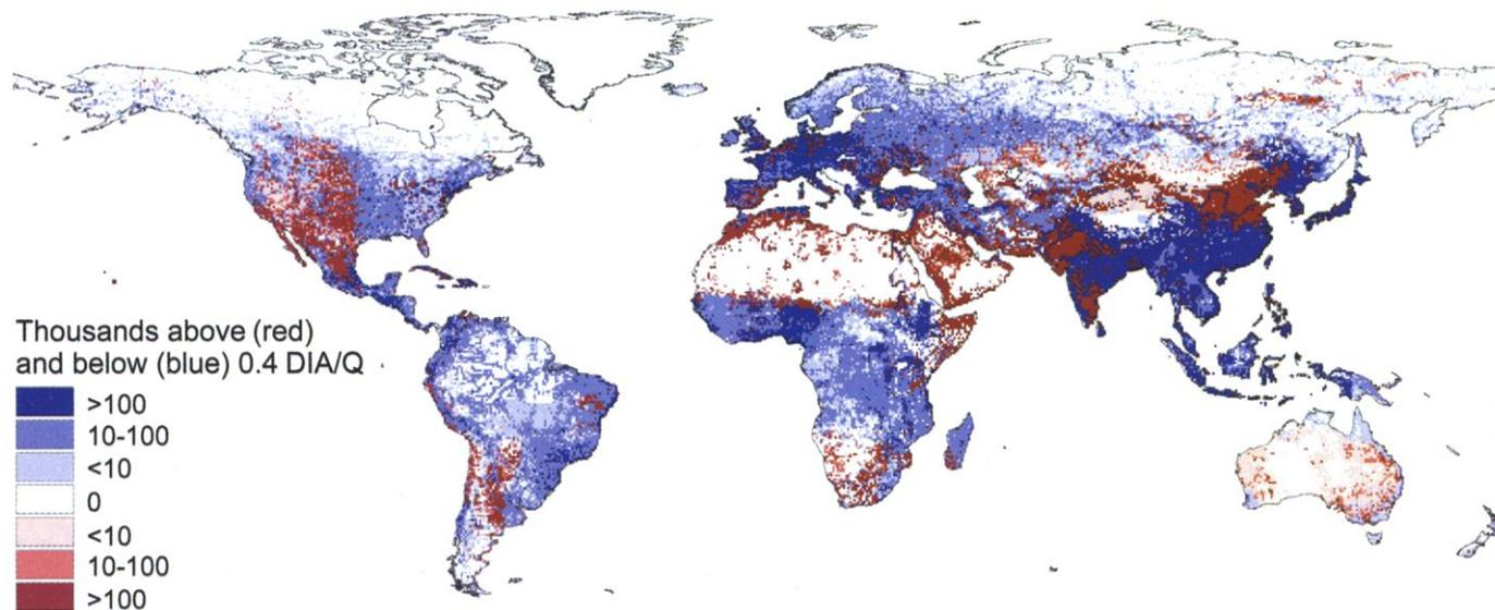
**Fig. 1.** The global distribution of population in 1985 with respect to the relative water stress threshold of  $DIA/Q = 0.4$  indicating severe water scarcity (10). A 30' spatial resolution is used. This mapping reflects a mean global runoff of  $\sim 40,000 \text{ km}^3 \text{ year}^{-1}$  and aggregate water withdrawals of  $3100 \text{ km}^3 \text{ year}^{-1}$ . These estimates are highly dependent on contemporary water use statistics,
