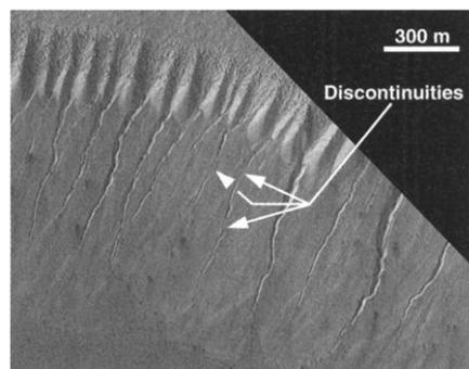
**Fig. 6.** Discontinuous reaches of some gullies (arrows) suggest that subsurface flow (or piping) may contribute to gully development. Illuminated from the upper left, this is a subframe of MOC image M03-02709, located at 70.8°S, 355.8°W.
