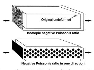
An unusual stretch. Stretching of materials with a negative Poisson's ratio causes an unexpected transverse expansion. This is unlike rubber and other common materials. If the material is isotropic, the expansion is in both transverse directions (top). Stretching cubic extreme matter can cause expansion in one direction and contraction in another direction at constant volume (bottom).
