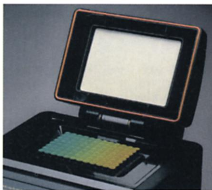
DNA Engine™, with the thermal gradient shown in artificial colors from data collected by an IR camera.
