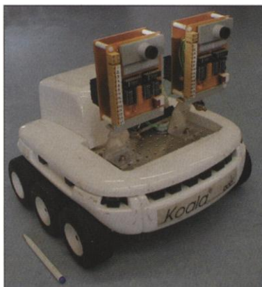
Picture of a neuromorphic "Koala" robot. Focal plane motion detector chips are mounted behind lenses on two boards, which carry additional discrete electronic components such as the trim potentiometers that set parameter voltages. Each chip has 37 elementary motion detectors. The aggregated outputs of the elementary motion detectors in each motion chip drive the motor system of the robot, and so generate the fly-like behaviors (optomotor response and fixation response).
