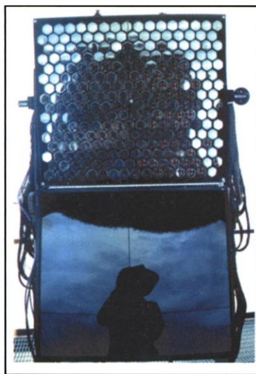
Fly specs. Clusters of phototubes give HiRes an eye for cosmic rays.
