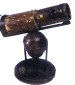
Reflector reconstructed. A reproduction of Newton's telescope from his original design.
