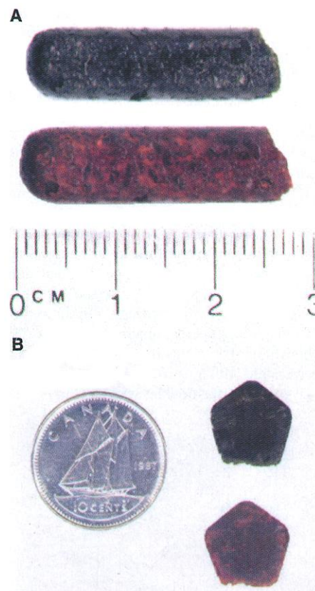
Fig. 3. (A) Photographs of the bulk organometallic polymer before (bottom) and after (top) pyrolysis at 600°C. (B) Photographs of the CPPN cast in a pentagonal Teflon mold before (bottom) and after (top) pyrolysis at 600°C. The ceramics retain the shape of the precursor polymer and show only a small contraction after pyrolysis (pyrolysis was not performed in a mold).
