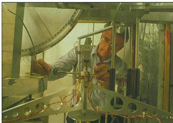
Walking the Planck. The heart of NIST's moving-coil watt balance, used to measure the Planck constant.
