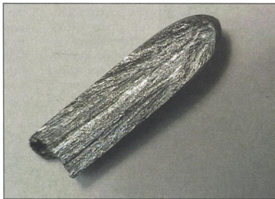
Chilly crystal. The new thermoelectric material carries away heat while it conducts electricity along its needlelike grains.
