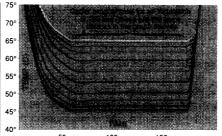
50 sec 100 sec 150 se Data from four cyclers are superposed in this graph, with each trace representing the average temperature measured in a column of wells. Note the consistency of incubation periods, the cycler-to-cycler reproducibility (each trace is made up of four separate lines), and the even spread of incubation temperatures between the programmed targets of 45° and 65°C.
