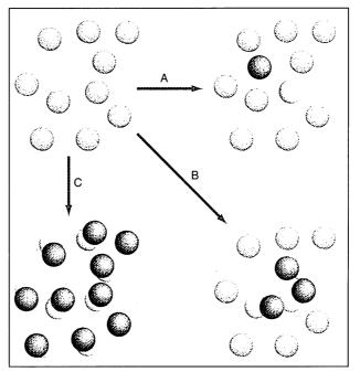
How do particles move near the glass transition? For each of the three possibilities shown, the average particle moves 20% of a particle diameter between frames. New particle positions are shown in red; vacated positions are pale red. Motion is either concentrated on one particle (A), or distributed across some (B) or all particles (C). Colloid motion is most like (C), but occurs primarily in a subset of unusually fast particles.
