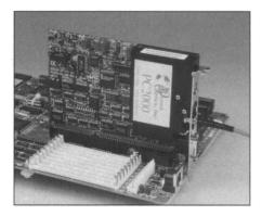
bench coupled to a high-sensitivity, 2048element charge coupled—device detector, and is especially useful for low light—level applications, such as fluorescence and plasma monitoring.
