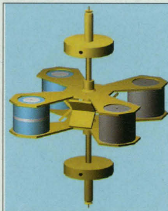
Earth (and moon) in the balance. Toy celestial bodies rest on a torsion balance, designed to detect differences in their response to the sun's gravity.
